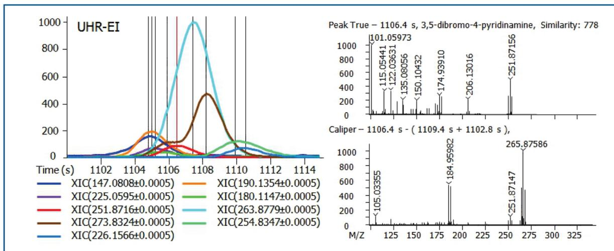
**Figure 2.** Extracted ion chromatograms of characteristic ions for nine peaks deconvolved using HRD. The deconvoluted (peak true) mass spectrum of the peak indicated with a red peak marker demonstrates the removal of background ions and other ions, such as masses from coeluting compounds that do not correspond to this dibromo-pyridinamine.
